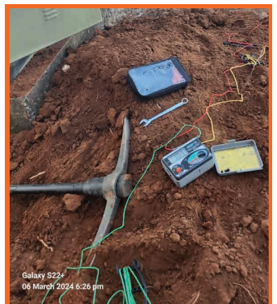
Combined Earthing results of Maintained 11kV ; 315kV ; 3Ph ; K3 Minisub at Goodhope Council Offices
