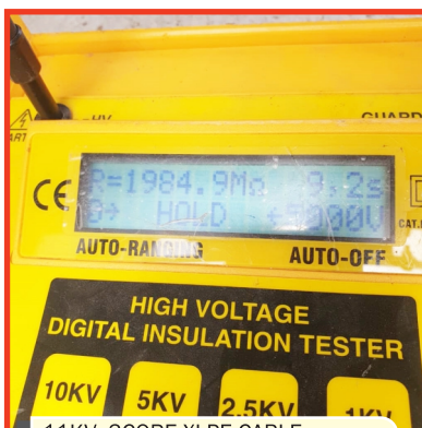
11KV; 3CORE XLPE CABLE UNDER TEST USING 10KV MEGGER
