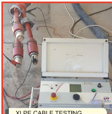
XLPE CABLE TESTING USING A VLF MACHINE
