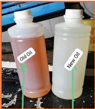
Transformer Oil Samples for testing . New oil was filled up in K3 Minisub at Goodhope Council
